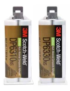
3M™ Scotch-Weld™ Multi-Material Composite Urethane Adhesive DP6310NS/DP6330NS is a two-part urethane adhesive that is used to bond most types of composites, metals and multiple materials together. DP6310NS is fast drying, with a 10-minute work time. DP6330NS allows a longer handling time of 30 minutes. It is designed to bond multiple applications and is ideal for bonding composites.
